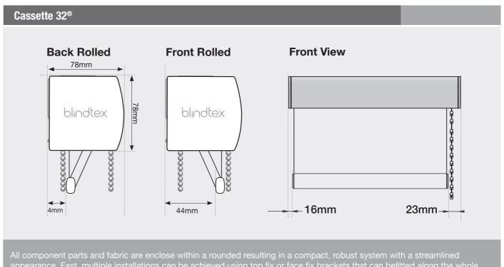
appearance. Fast, multiple installations can be achieved using top fix or face fix brackets that can befitted along the whole ength of the cassette. The snap fix fascia can be white, cream, grey or black or with a matching fabric profile.
