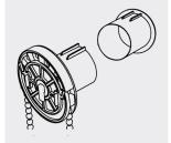
Side action control unit & plunger in engineered plastic. Unit locks into brackets. Clutch type suitable up to 9kg weight. Can be left or right control.
