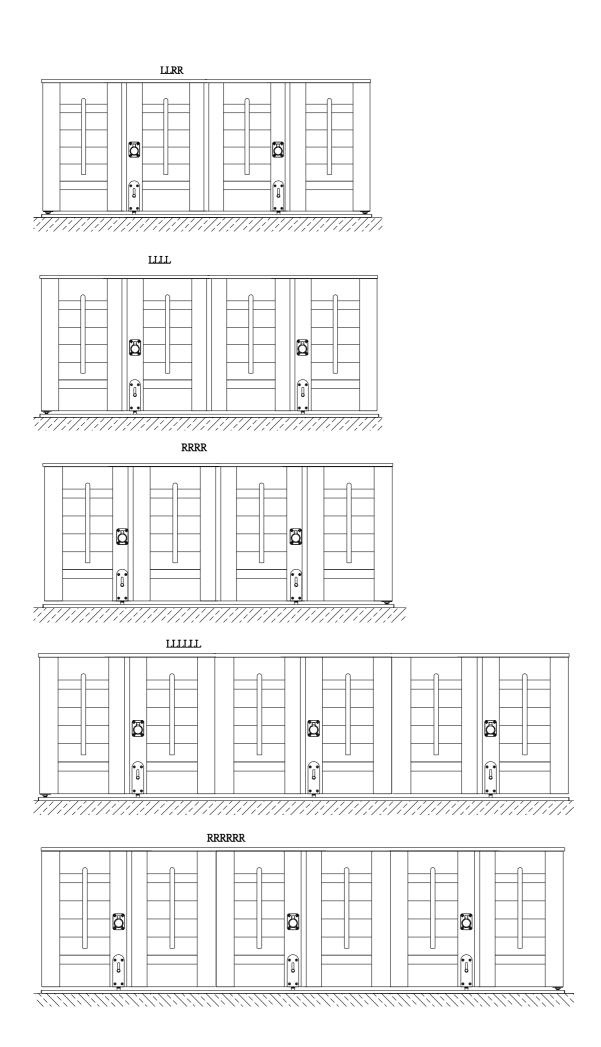
The bolt location for both track system shutters and regular shutters would be the same.
